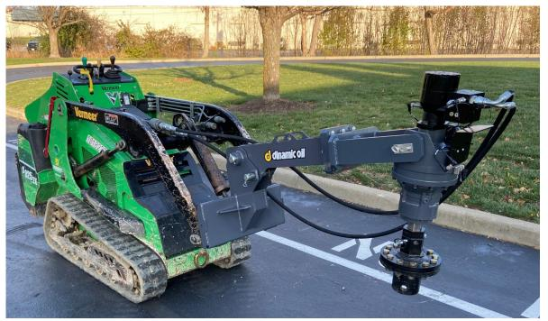
Leveraging the multiposition feature of the mini-mount can quickly reduce setup/tear-down time and decrease transportation costs.
