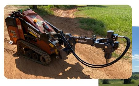
Designed for universal mini-skid loader quick attach and Bobcat® Bob-Tach® systems.
