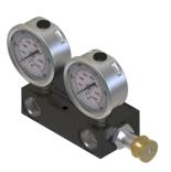
The Pressure Relief and Differential Kit (PRDK) provides the ability to monitor and calculate the differential pressure being applied to the Anchor Drive. Two liquid-filled gauges mounted an aluminum block with relief valve can be used with any prime mover and make/model of Anchor Drive. Available for applications up to 3000 PSI.
