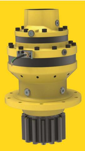
Dinamic Oil's new *Torque Detection System* provides real-time torque feedback from within the gearbox, thus eliminating the uncertainties and errors inherent to pressure-based or external load cell designs. Strategically placed strain gauges inside an intermediate flange offer accurate and repeatable results while still maintaining the same overall dimensions as a standard gearbox.
